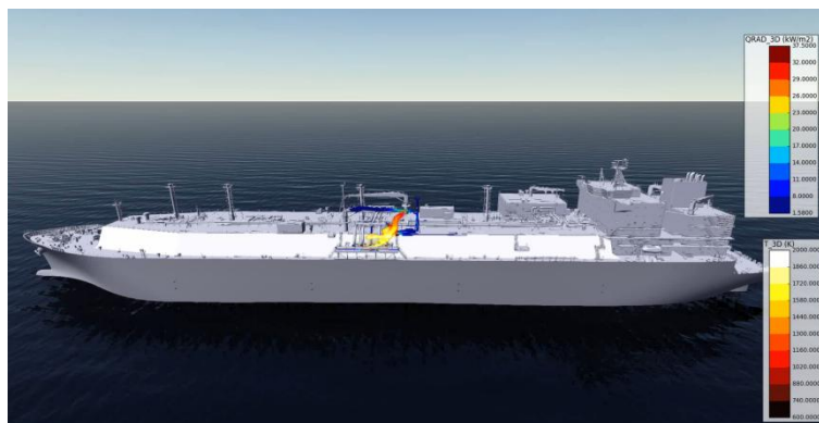
Fig. 2.6-2 Fire diffusion after jet leakage
